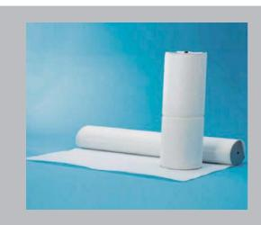
Filtering septum in AT/R210 series resin-bonded and laminated synthetic polyester fibre with support in treated polyester mesh with a basis weight of 210 g/m² and a thickness of 10 mm. The adhesive resin on the material and the fibre structure ensure high dust collection and retention efficiency. The length of the filter mat is 15 lm. The core around which the filter mat is wrapped consists of a hollow galvanised steel tube (cardboard core on request).
